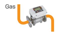
The flow meter has to be located 10D or more distant from a governor irrespective whether it is placed upstream or downstream of the governor. Falling to meet this condition may lead to inaccurate measurements, (D = pipe diameter)
