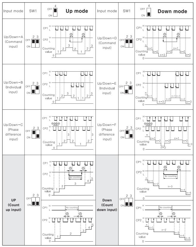
**※**❷ : Over Min. signal width, ❸: Over 1/2 of Min. signal width.
