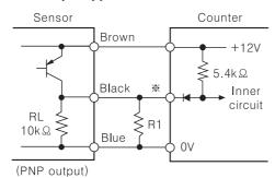
•Please set R1 value to make the composed resistance of RL + R1 as Max.  $470k\Omega$  is an impedance for short-circuit.
