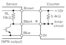
Brown +12V  $5.4k\Omega$ Black Inner circuit Blue 0V (NPN open collector output)
