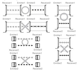
Shield panel should be installed between 2 sets >
