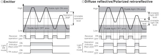
☀The waveform of 'Operation mode indicator' and 'TR output' is for Light ON mode, it is operated as reverse in Dark ON mode.
