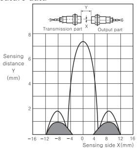
Please note the proximity sensor detects the surrounding cover of the sensing side of transmission coupler even the connection switch is OFF. (Sensing part) for ■ part.
