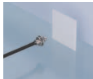
Sensor turns ON when the target enters the sensing area
