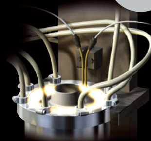
Management of cooling water flow volume for high-frequency hardening equipment.
