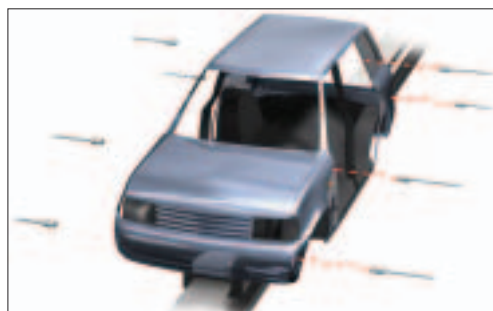
Checking the passage of cars on a conveyor. Sensor used: PX-H72G.
