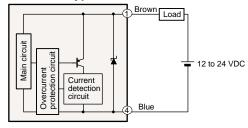
\* The M8 sensor does not contain short-circuit protection or a current detection circuit. (1) and (4) in the circuit diagram shows the pin number of the connector type.
