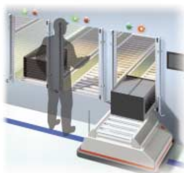
Worker penetration is prevented at a row of parallel pickup windows.
