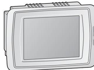
The **E1012**, **E1022** and **E1032** have programmable function keys and a separate keypad. The graphic-capable displays illustrate symbols, alarms, line diagrams and text in arbitrary sizes. Formulas, text and changes in the sequence program can be done directly via the keys.
