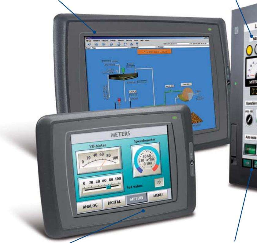
Units with high IP ratings ensure easy and carefree cleaning, especially useful for situations that require full wash downs.
