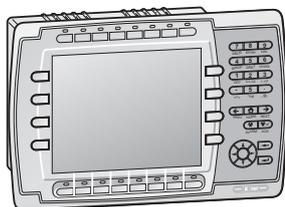
The operator terminal **E1070** offers a 6.5" TFT display with 65,536 colours and a resolution of 640x480 pixels. 16 freely programmable function keys facilitate the inputs directly at the terminal.
