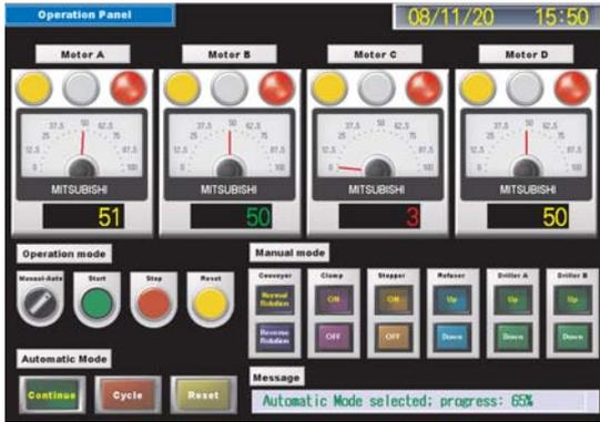
Advanced screen design software such as GT Designer enable screens to be quickly and efficiently created.
