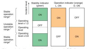
\*If the operating level is set to the stable operation range, the E3G will operate with the highest reliability and without being influenced by temperature change, voltage fluctuation, dust, or setting change. If the operating level cannot be set to the stable operation range, pay close attention to environmental changes while operating the E3G.
