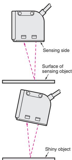
If detecting a shiny object, however, mount the Sensor so that the sensing face is at an angle of between 5° and 10° of the surface of the object being detected as shown below, and check to be sure that there is no interference from the background.
