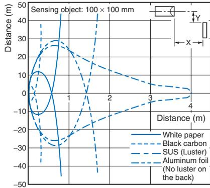
**Sensing Object Size vs. Sensing Distance**
