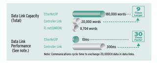
Using the CJ2H built-in EtherNet/IP port (Functionality differs when using the CJ2M built-in EtherNet/IP port)
