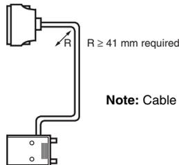
**Note:** Cable thickness: 5.1 mm dia.
