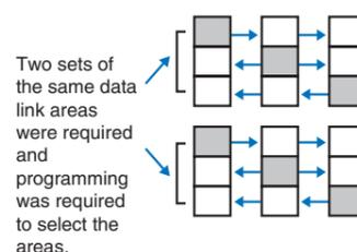
Just create the data links for one Controller Link Unit to eliminate wasted data memory. The Duplex Controller Link Units share the data links.
