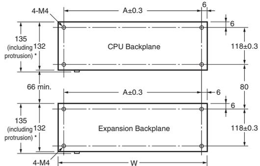
\* The CS1D Backplane has no protrusions.
