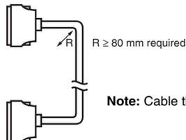
**Note:** Cable thickness: 10 mm dia.
