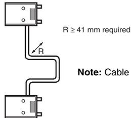
**Note:** Cable thickness: 5.1 mm dia.
