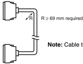
**Note:** Cable thickness: 8.6 mm dia.
