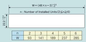
Vertically Consecutive Installation in One Hole (Max.6 units) Non-application of IP66
