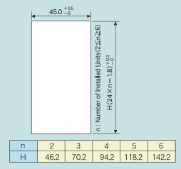
Metal fittings are needed for each unit in case of vertically consecutive installation in one hole.
